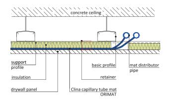
View of a ceiling section: jointless drywall ceiling with capillary tube mat
