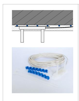
Before plastering the ceiling, attach the dew point sensor to the flow of the capillary tube mat, this means as close as possible to the mat distributor pipe.
