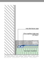
View of a floor section: capillary tube mat in screed
